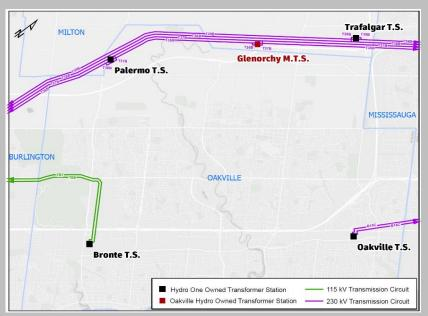
Figure 1: Transmission Connections - Oakville Hydro
